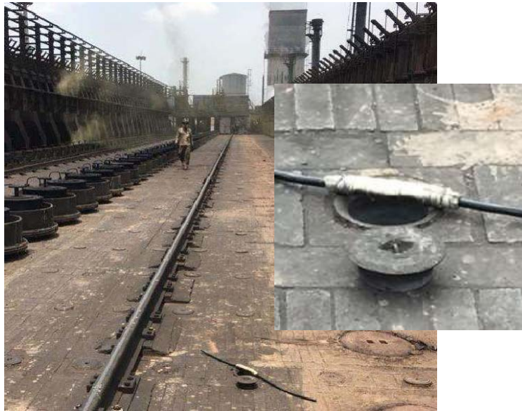
Kept on Coke Oven battery area on Top at Temperature greater than 300 deg C
