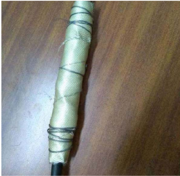
Hi-Temp Tape wrapped on a cable
